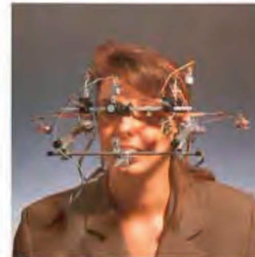
Fig 3 Electronic pantography: facial arcs mounted for recording mandibular movements.
